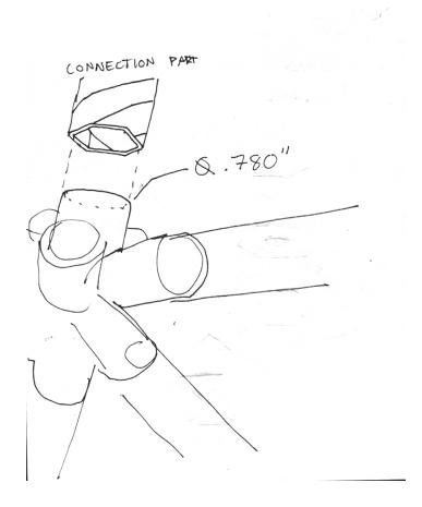
While working with paper and resin, I discovered that I could make paper tubes made up of 3 wound layers. The direction of each winding opposed the one beneath it to make a cross grain effect. I decided that this would be a good initial material to create
