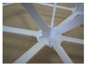
While designing the building system made of paper tubes, I was also designing a second system. This system is cut from sheet stock and uses no hardware. It forms the same tetrahedral structure. The spars press fit into the nodes and are held in place by teeth.
